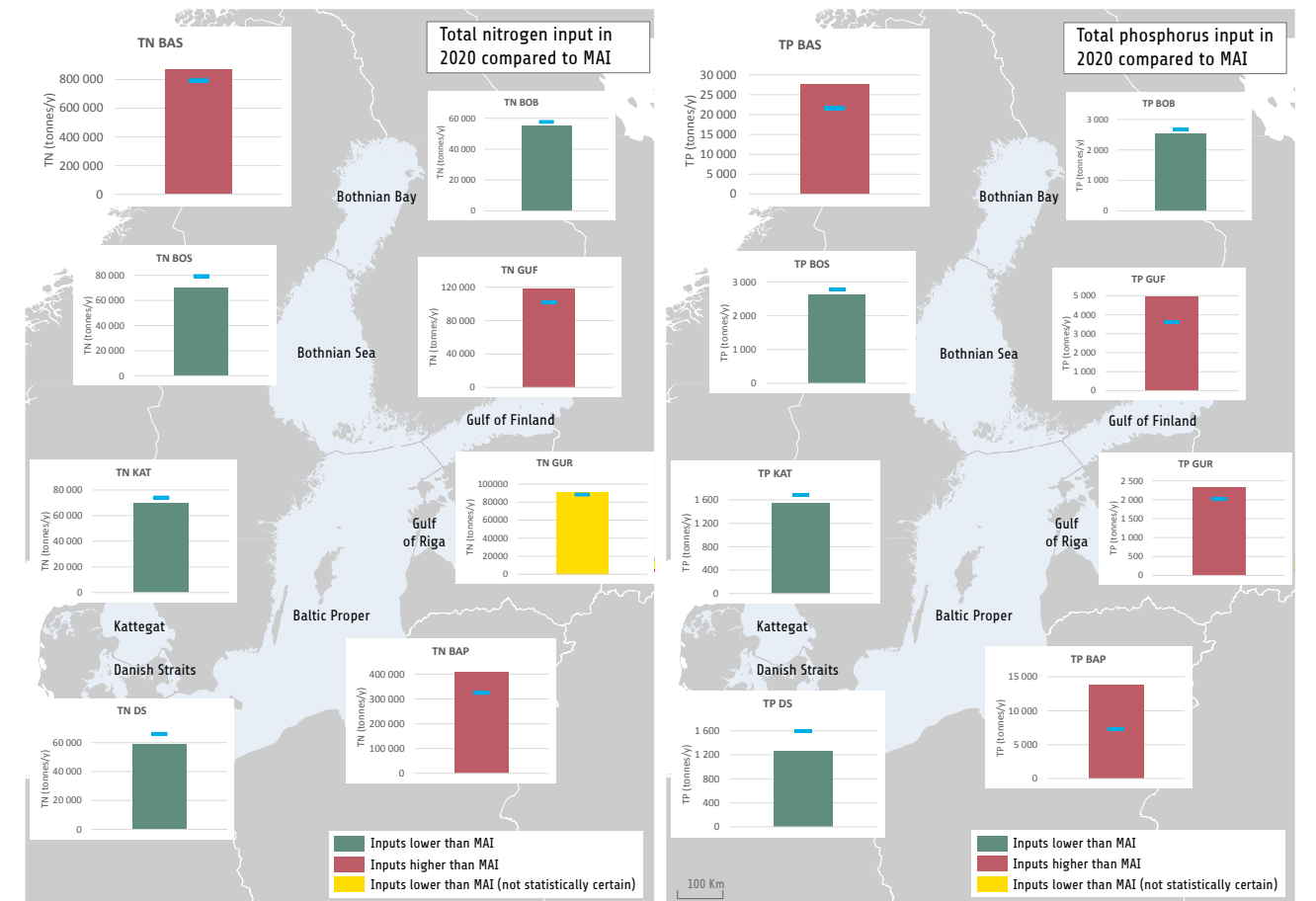
Figure 4.5. Inputs of nitrogen (left) and phosphorus (right) to the Baltic Sea sub-basins, as these are defined in the HELCOM pollution load compilation. BAS=whole Baltic Sea. The columns show trend-based estimates of total nitrogen and phosphorus inputs in 2020, in tons per year and including statistical uncertainty. The short blue lines show the maximum allowable inputs (MAI). Green indicates that the estimated inputs, including uncertainty, were lower than MAI, while red indicates that they exceeded MAI. Yellow indicates that the statistical uncertainty of the input data makes it not possible to determine whether MAI was fulfilled. Note that the scale of the y-axis differs between charts. Source: HELCOM 2023f.
